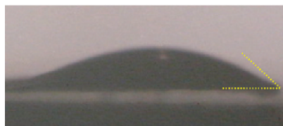
FIGURE 7. Contact-angle measurement images of (left) SPIO-NH 2 - and (right) SPIO-G2-Zn-coated mica surfaces.
